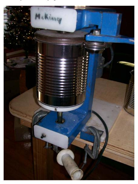
Now press the button that makes the can spin around. There's a handle at the top of the unit that crimps the lid over the flared top of the can. The instructions state to pull the handle for three rotations of the can the push the handle for three rotations.
