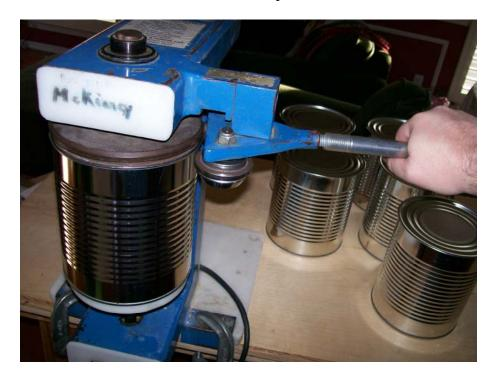
It's difficult to see from this picture, but there is a second "wheel" on the back side of the unit that engages when you push the handle.
